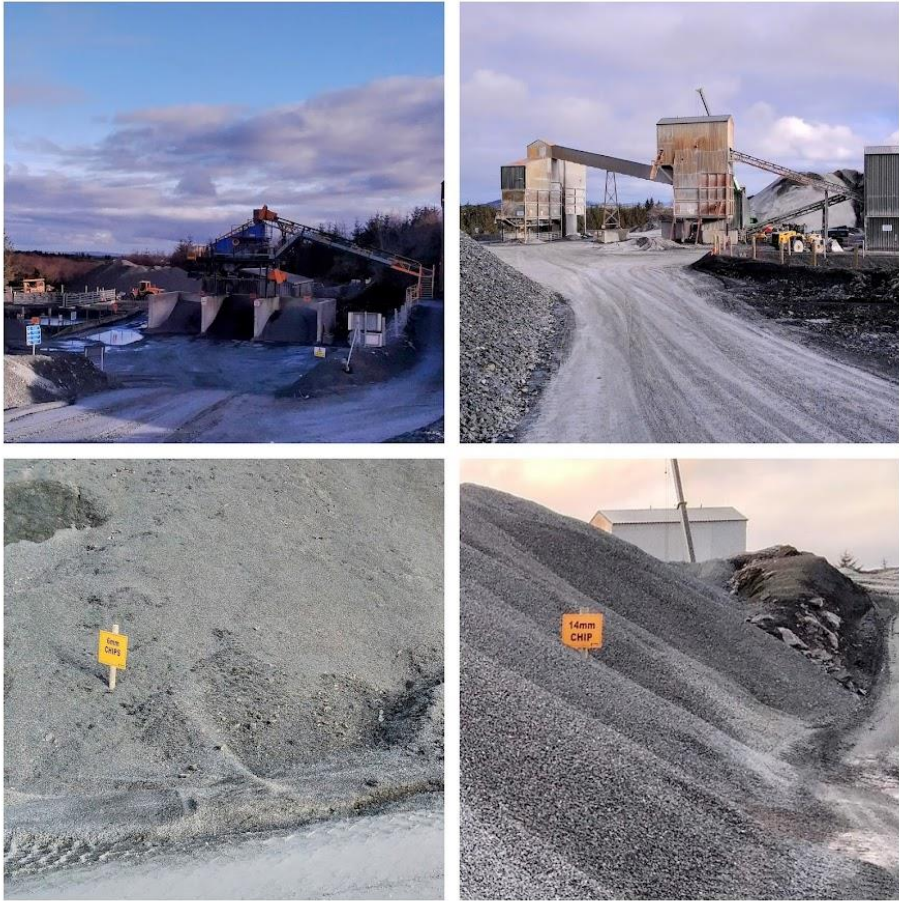
Segregation and labelling of aggregate stockpiles
